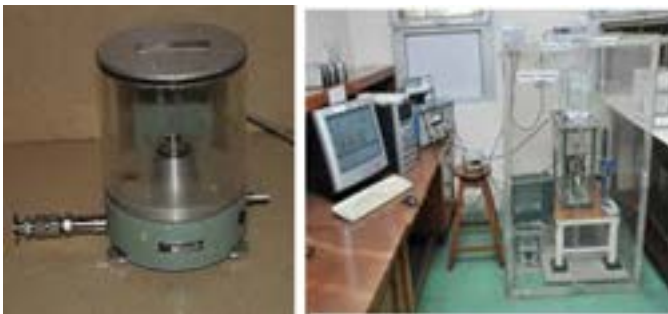
Secondary standard for Pneumatic pressure measurement and Primary standard for ultrasonic power measurements
