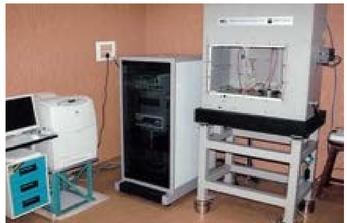
The first Iodine frequency stabilized He-Ne Laser at NPL, used for realization of metre and Automatic Gauge Block Interferometer, first link between definition of unit metre and length measuring artifacts - Gauge Blocks used to disseminate traceability to various upto 300 mm
