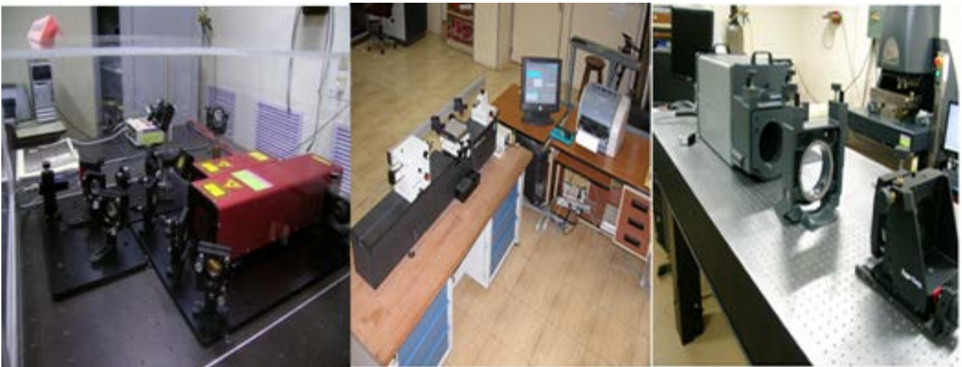
Current Primary standard of length, Length measuring machine and Flatness measuring interferometer
