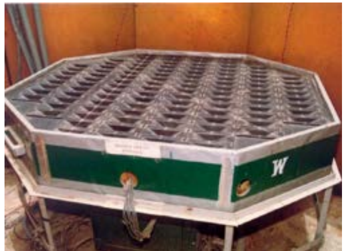
Initial stages of Sodar antenna development at NPL and Phased array wind profiling Sodar
