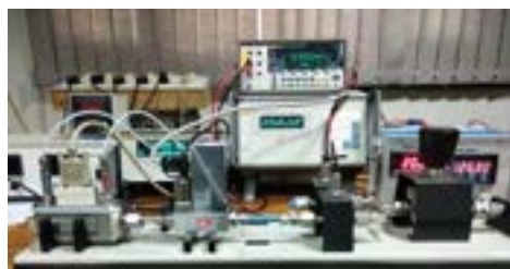
(a) Set-up for calibration of Mass Flow Controllers
