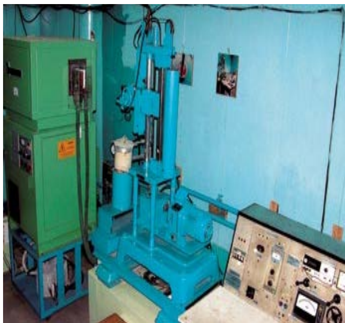
In house developed Czochralski crystal puller
