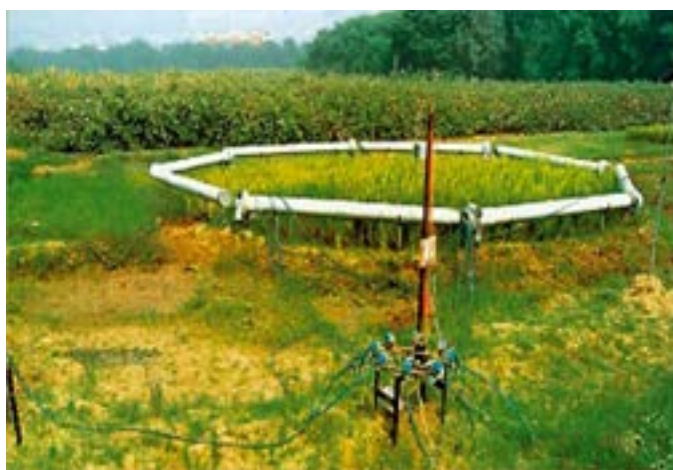
An automatic facility to enhance CO 2 in the open air was developed by CSIR-NPL and installed at IARI campus, New Delhi
