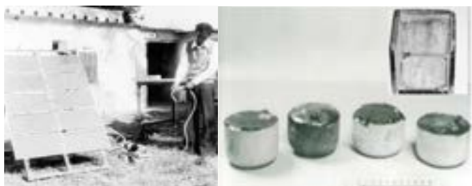
Demonstration of water pumping using indigenously developed 16 mm size polycrystalline silicon solar cells at NPL; Reusable graphite crucible used a number of times to grow multi-crystalline silicon ingots
