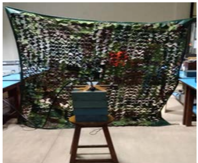
RF transparency measurement using open air antenna method for X- band Frequencies (Front and back view)
