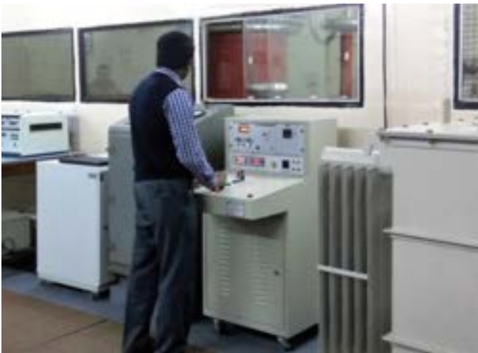
Measurement set-up and Control Unit for AC High Voltage Source
