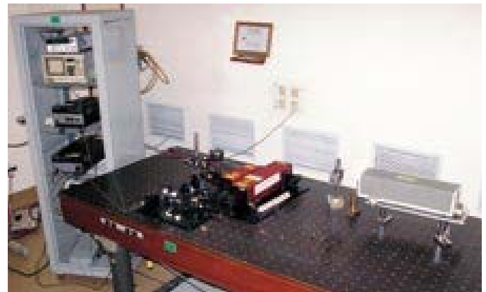
The ultrasonic Interferometer Manometer for absolute low pressure measurement and the Primary standard for hydraulic pressures upto 1 GPa;
