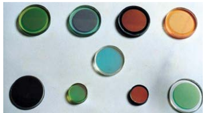
Various types of interference filter coatings developed at NPL
