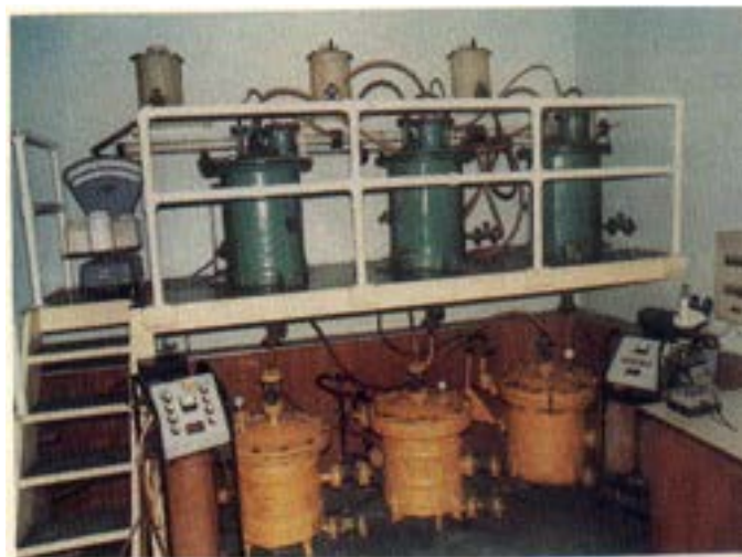
Pilot plant created for production of ZnS based color TV phosphors at NPL
