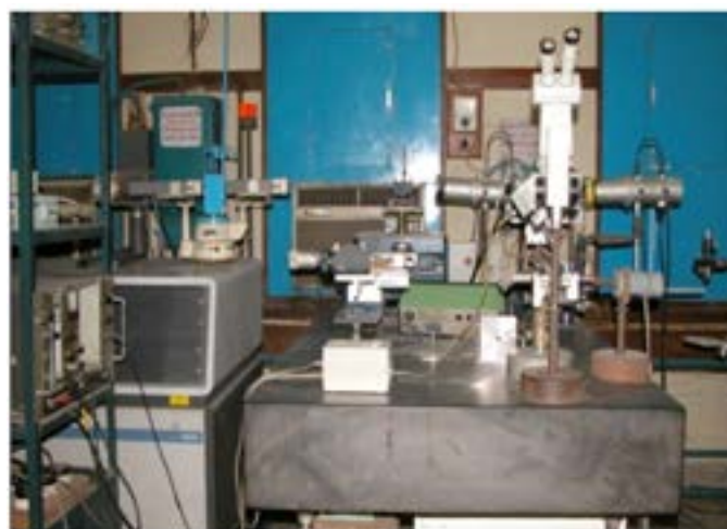
Photograph of the multi-crystal X-ray diffractometer designed, developed and fabricated at CSIR-NPL.
