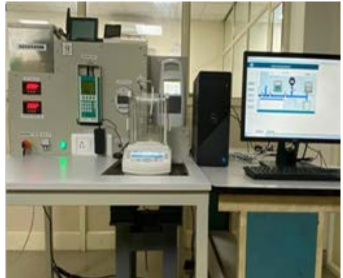
Calibration facility for defibrillator & defibrillator analyser and calibration set-up for Infusion pump device/ infusion pump analyser at CSIR NPL
