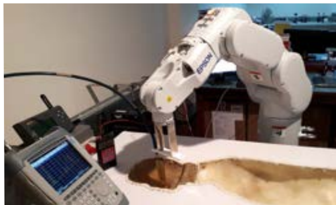
SAR set-up, E-field sensor with robotic automation
