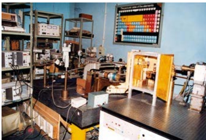
Photograph of Five Crystal X-ray diffractometer designed, developed and fabricated at CSIR-NPL.
