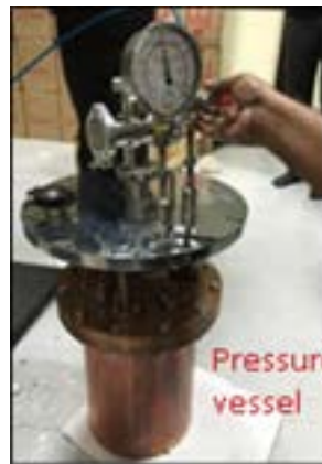
Mirror Polished Copper Quasi Resonator, pressure vessel and vacuum vessel for realization of Boltzmann constant k
