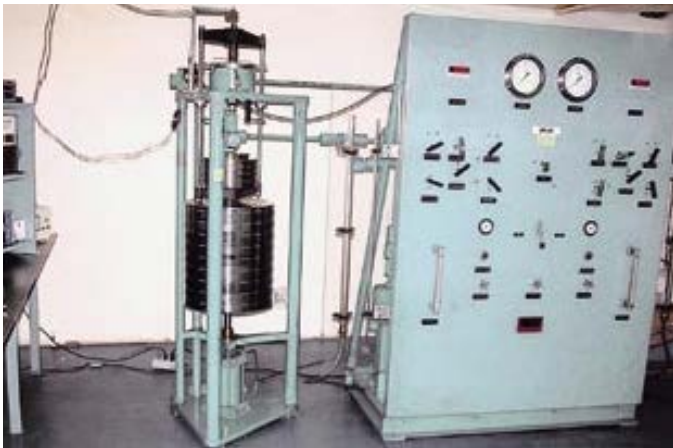
The ultrasonic Interferometer Manometer for absolute low pressure measurement and the Primary standard for hydraulic pressures upto 1 GPa;
