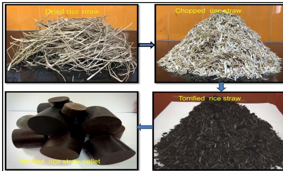
Dried Rice Straw, Chopped Rice Straw, Torrified Rice Straw Product and Pellet from different Torrified Products
