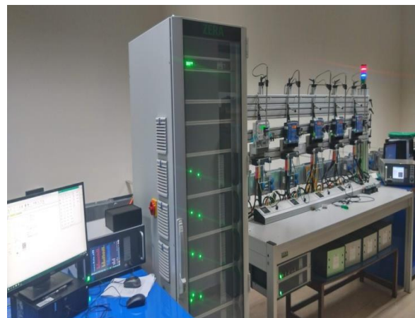
AC Power & Energy Calibration and Test
