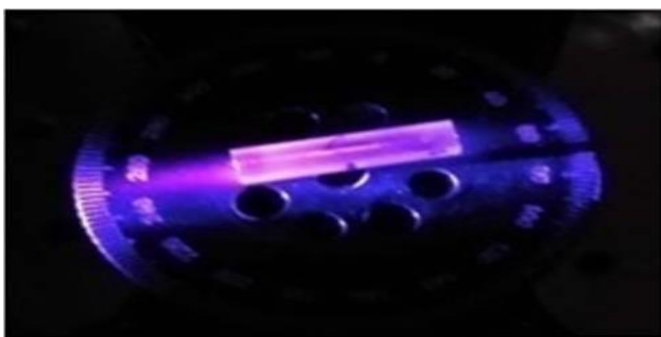
Blue Laser Emission at 457nm using BBO/LBO crystals
