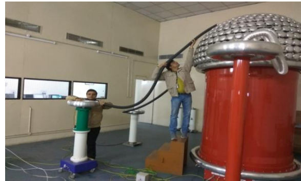
AC High Voltage Calibration Setup
