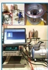
Device developed for the testing of thin films sensor for air pollutant gases
