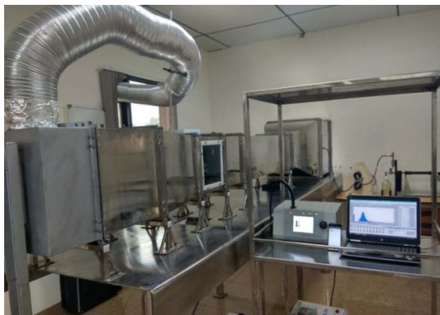
Indigenous Developed Wind-tunnel Facility to Test and Calibrate PM 1 , PM 2.5 and PM 10 Samplers
