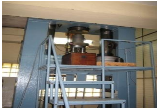
3 MN Build-up System for Force
