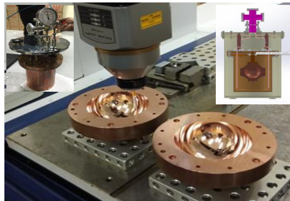
CMM Measurements on Diamond Turned Hemispheres of Copper Cavity Resonator Developed to Realize Boltzmann Constant based New Kelvin
