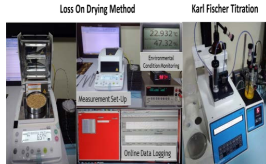
Moisture Measurement Set-up based on Loss-on-drying Oven and Karl Fischer Titrator
