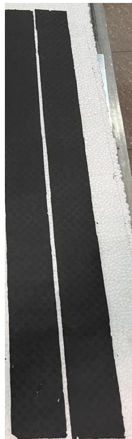
CNT Paper strips of 60 mm width and 70 cm length
